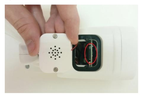
3. Insert SD card (golden pins facing the top of the camera).
