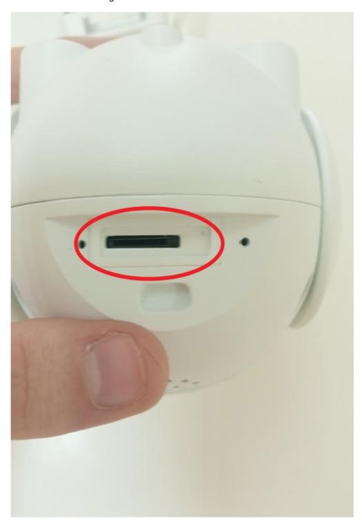
3. Insert SD card (golden pins facing camera speaker) assemble SD card flap and screw it to the body of the camera.
