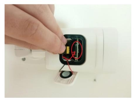
4. Assemble the SD card flap and screw it to the camera body, remember to screw flap on with the dot facing towards camera holder.
