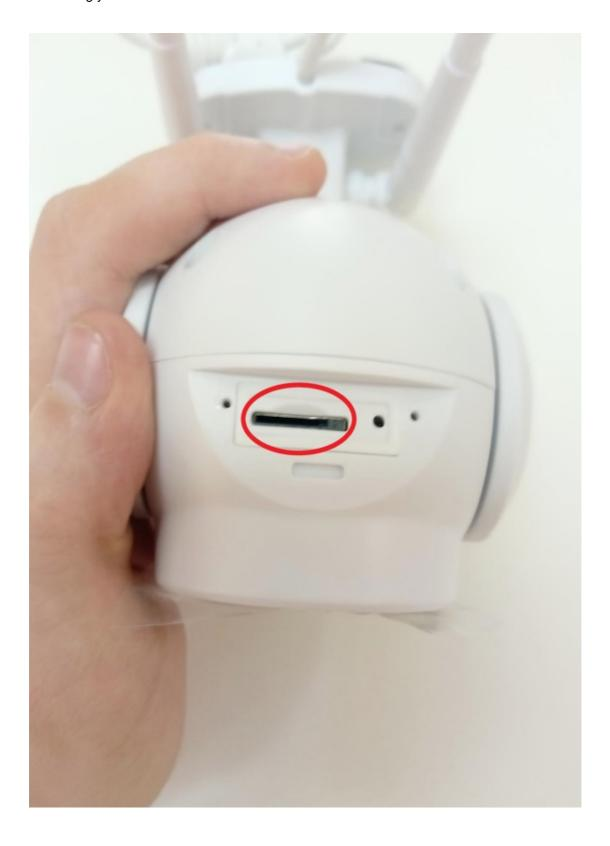
3. Insert SD (golden pins facing eye of the camera).
